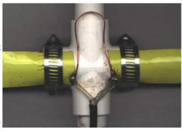
Figure 1 shows the method used to attach the driven element to the PVC cross.
