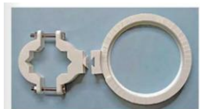
Figure 3 — A 3D-printed mounting bracket for a large balun attached to an end cap with #10-24 × 1-inch stainless-steel screws.
