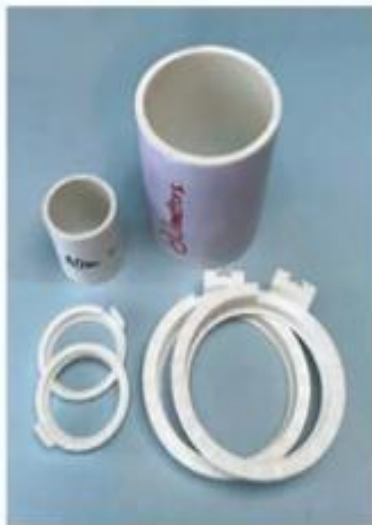
Figure 1 — End caps and body pipes. Note ramps on rings to keep turns together.
